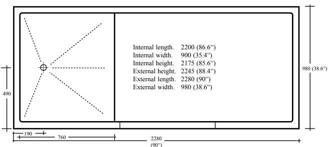
Includes; FP1000S Bathroom Module. Chrome shower and basin mixers, full ceramic toilet suite, wall mounted ceramic basin with plug & waste, shower floor waste fitting, mirror, towel rail, toilet roll holder, soap dish. All fittings are supplied loose ready for site assembly. Installation on site is not included. Prices are ex factory. Limited stock available, units are in smooth finish, colour is White w/ white sanitary ware.
